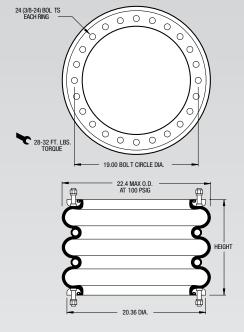
NOTE: A bead ring part is shown. This part is also available with rolled plates. See page 11 for explanation.
